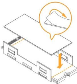
4. Align the heatsink to the edge of the bracket and press down the heatsink into the bracket until it clips into place.
