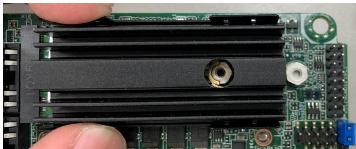
For M.2 2260 module, you could lock the screw directly.
