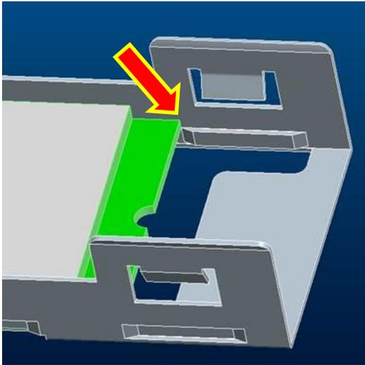
3. Remove the membranes from both sides of the thermal pad firstly, and then paste the thermal pad onto the M.2 module. If you used M.2 2242 module, please cut the thermal pad to a suitable length to cover M.2 2242 module.
