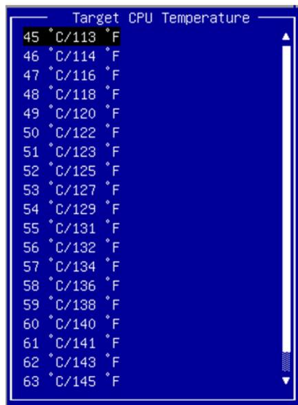
If CPU temp is lower than target temp, the fan will run at target fan speed.
