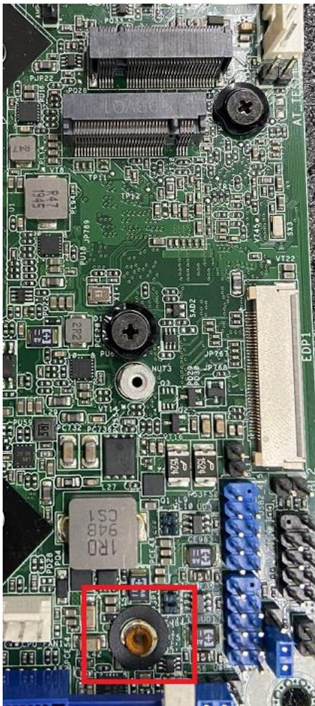
2. Vertically use the Hexagon socket screwdriver to release the standoff counterclockwise.
