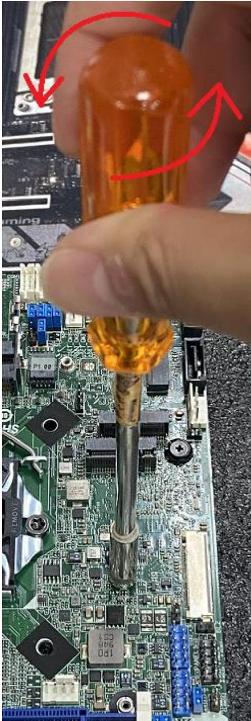
3. Vertically use the Hexagon socket screwdriver to fasten the standoff into the M.2 device screw hole clockwise.
